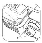
Disconnect the spark plug lead.
